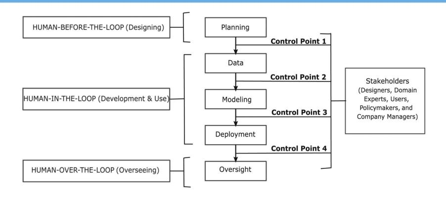
Different levels of human involvement and different control points that can be used for better controllability and checking in the development of trustworthy AI.
